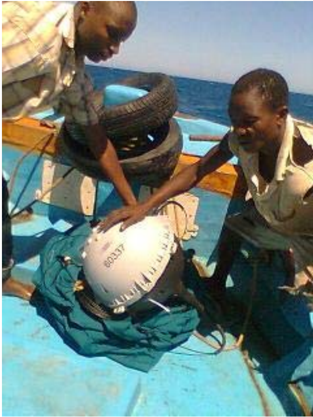
Plate 1: View of an Argo drifter in preparation for deployment in between the mainland and islands in Sofala Bank, December 2007.
